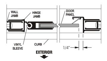
Inside the shower enclosure, drill two 1/8" holes thru the hinge jamb and into the wall jamb [C] 3/8" to 3/4" from the wall and approximately 1" vertically from each end of the hinge jamb. Drill a third hole centered between the first two, then enlarge the three outer holes with a 3/16" drill for clearance on the selftapping screws. Attach the door panel assembly permanently with three  $\#6 \times 3/8$ " pan head screws [**F**].
