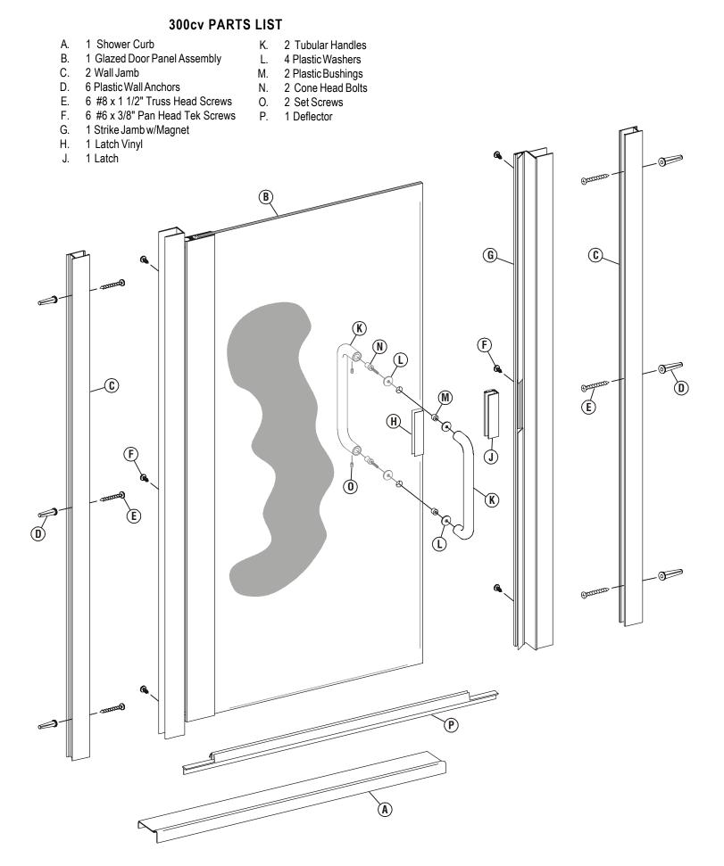
The Alumax 300cv Continous Hinge Shower Door is completely reversible and may be installed hinge-left or hinge-right. Refer to the illustration to determine the correct position for your installation. For maximum waterproofing, the hinge jamb should always be opposite the shower head. These instructions depict a hinge-left installation.
